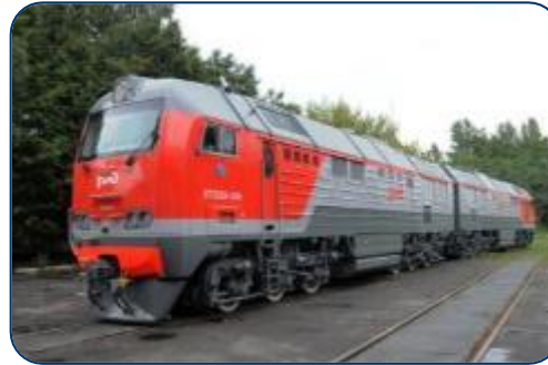
2TE25A 'Vityaz' with asynchronous traction motors
