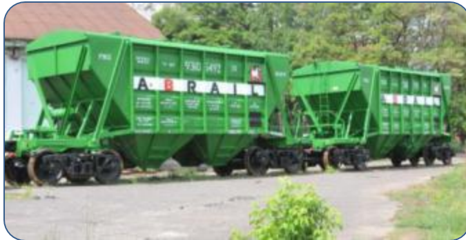
19-3018 model hopper wagon for cement transportation
