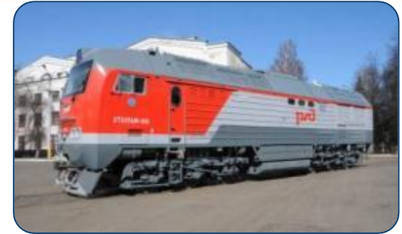
2TE25AM with asynchronous traction motors
