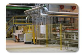
Capacity of short-cycling presses allow to laminate all chip board from two main presses
