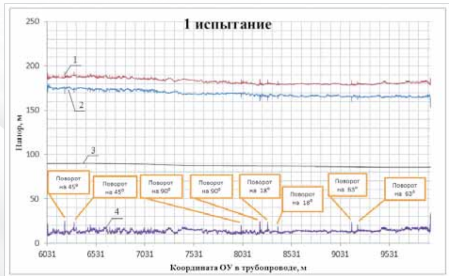
Cleaning pig’s pressure loss in passing through the pipeline turns in the segment between the valves 33 and 34 (6031 – 9954 m).
